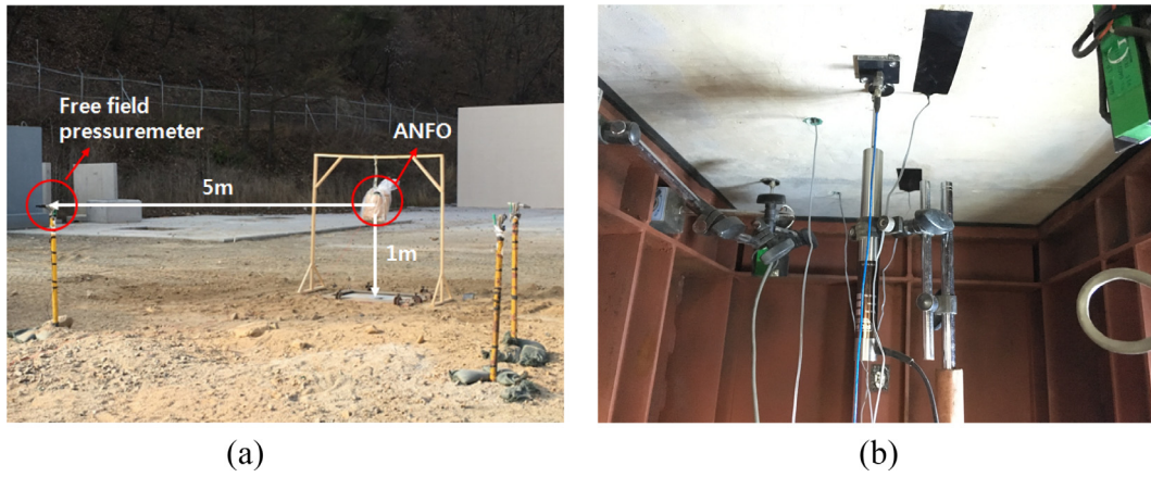
Fig. 8. Overall blast test setup and measurement equipment photos: (a) Placed concrete specimen; (b) LVDT.
